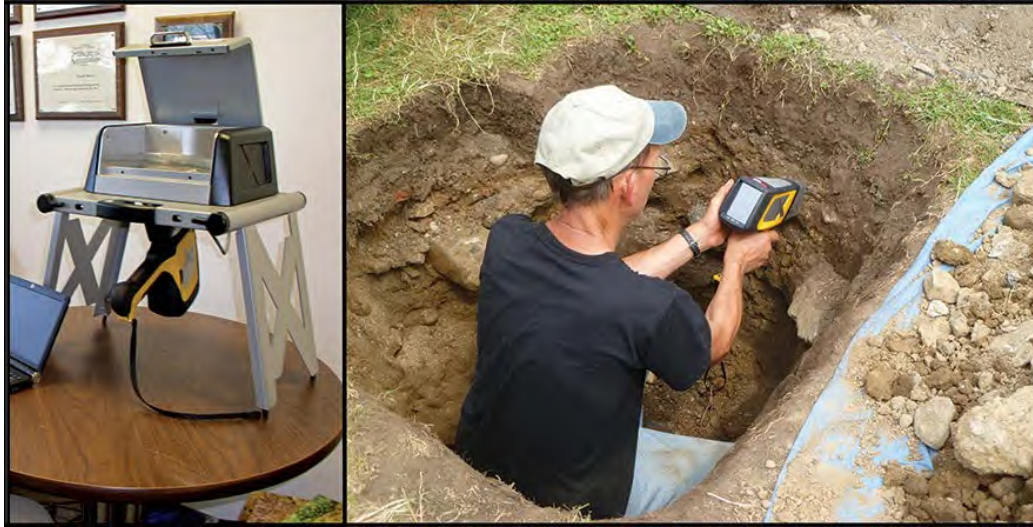
A portable XRF spectrometer, which can be attached to a monitoring bench in an office to scan collected samples (left) or can be used in the field to scan exposed faces of soil pits or surfaces (right).
