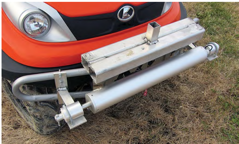
A vehicle-mounted passive gamma-ray sensor.
